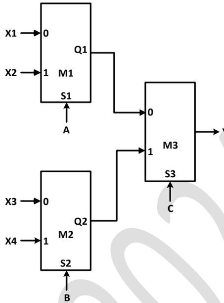
For an instance of inputs  $X1=1$ ,  $X2=1$ ,  $X3=0$ , and  $X4=0$ , the number of combinations of A, B, C that give the output  $Y=1$  is \_\_\_\_\_
